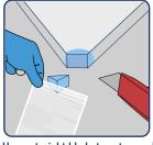
Use a straight blade to cut a small sample. Do not use a serrated edge or disturb the material any more than is needed.
