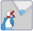
Fill a spray bottle and use a fine mist to wet the sample in order to reduce airborne fiber release.
