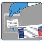
Place sample in resealable bag. Fill out the label and fill in Chain of Custody form or go to website.
