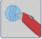
It is important to remove all layers of paint when collecting the sample. Older layers are what usually contain any lead.
