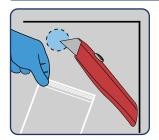
Use a straight edge blade to cut a small sample piece no smaller than the size of a quarter. Do not use a serrated edge.
