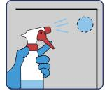
Fill a spray bottle and use a fine mist to wet the sample in order to reduce airborne dust and debris.
